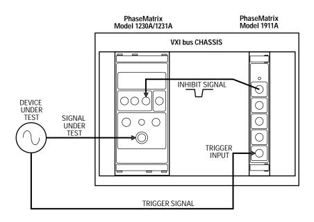
This simple setup can fully characterize time varying microwave frequencies quickly and accurately
